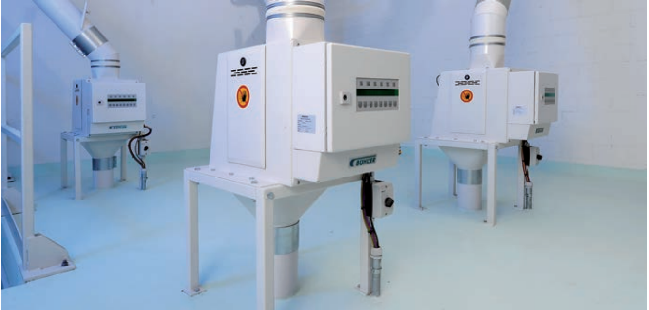
Flowbalancer MZA.H. for an optimal blending of grain varieties.
